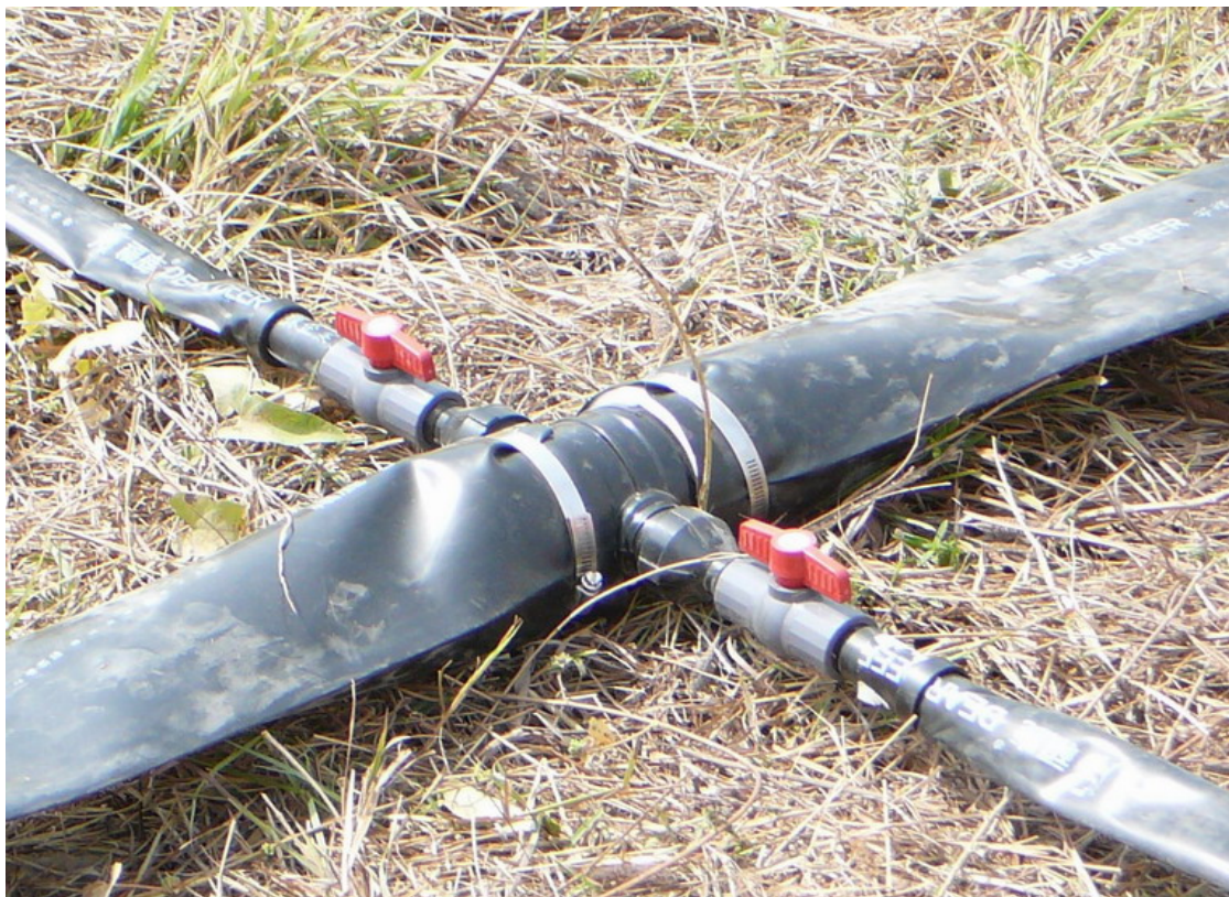
Main pipe is flexible flat hose
