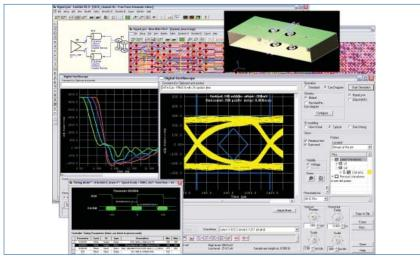
HyperLynx SI includes tools for pre- and post-layout signal integrity, timing, crosstalk, and EMC analysis, for signals ranging from 0 Hz to multi-GHz.
