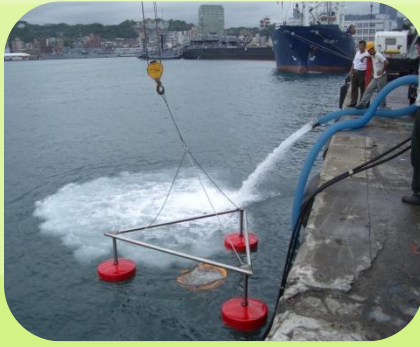
外海堰式汲油器(250m 3 /hr) Weir Skimmer
