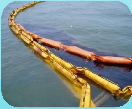
圓筒型固體填充式攔油索 Fence Boom (Column)
