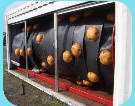
永久固定式攔油索 Permanent Containment Boom
