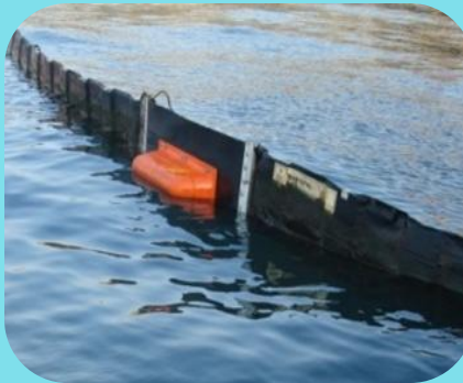
永久固定式攔油索 Permanent Containment Boom
