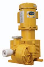
AquFlow Series 2000 metering pump is a compact pump designed for its accuracy and durability. Its hydraulically balanced design means the life of its components including the diaphragm is long lasting. The wear is minimised on all its drive parts by enclosing it in an oil bath. The wetted components for the pump are available in various materials to assure compatibility with tough chemicals (refer to the Material Selection table on the following page)
