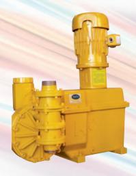
The AquFlow Series 4000 is a rugged, durable, hydraulically actuated and balanced diaphragm metering pump. The pump is available in simplex or duplex configuration, with independent capacity adjustment for each pumphead.
