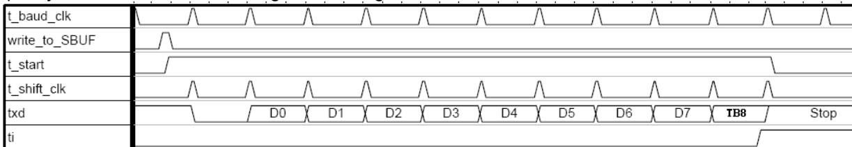
Fig. 8-5: Transmit modes 2 and 3
