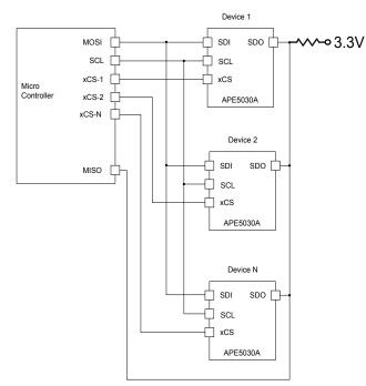
Figure 8: SPI Parallel Structure
