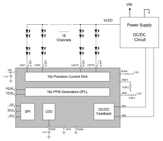
Note:When LED1 to 16 of APE5030A pin-out location to external LED string cathode location has execcd 1uH wire inducutance, suggestion add the MLCC capcitors for holdout interference.
