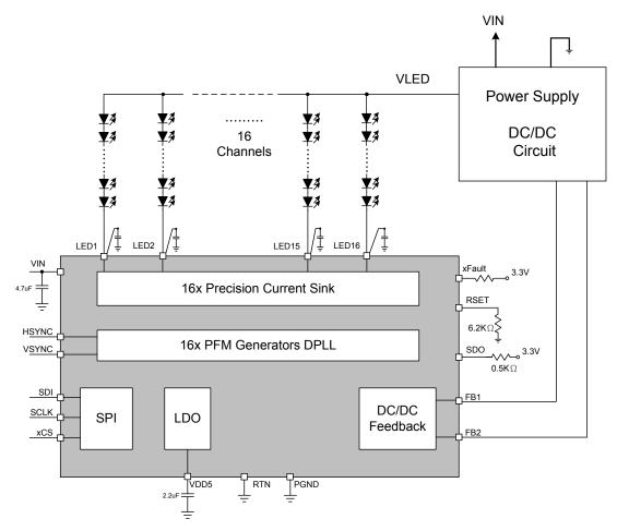
Note 4:When LED1 to 16 of APE5030A pin-out location to external LED string cathode location has execcd 1uH wire inducutance, suggestion add the MLCC capcitors for holdout interference.
