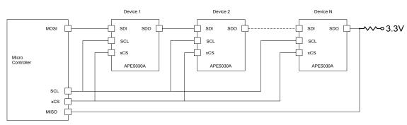
Figure 7: SPI Daisy Chain structure
