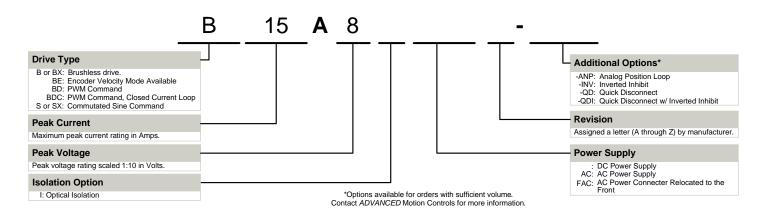
ADVANCED Motion Controls analog series of servo drives are available in many configurations. All models listed in the selection tables of the website are readily available, standard product offerings.
