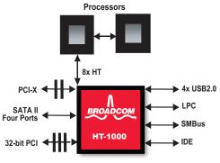
HT-1000 Connected Directly to Processors
