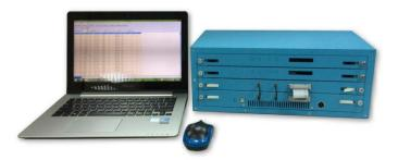
LT2000E Touch Panel Tester is designed to test the touch sensor electrical characteristic using.LT2000E can test touch sensor's Open, Short, Wire resistance, Insulation resistance and Node capacitance, which can measure the Insulation resistance to 1000M ohm, and Node capacitance can be measured to 0.1 pF.
