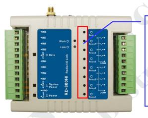
When RD-800HI receives controlling signal to drive the relay movement, the corresponding relay indicator light will follow the relay movement to glimmer or keep being bright.
