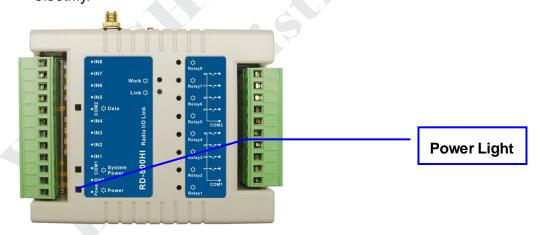
• System Power Light: When the indicator light keep being bright, it means the each working voltage is no problem.
