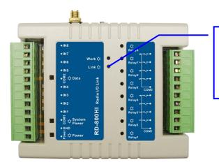
When RD-800HI link to the settle group in working range, the link indicator will keep being bright.
