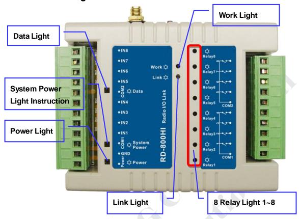
• Power Light: When the light is bright, it means the device is opened and to electrify.
