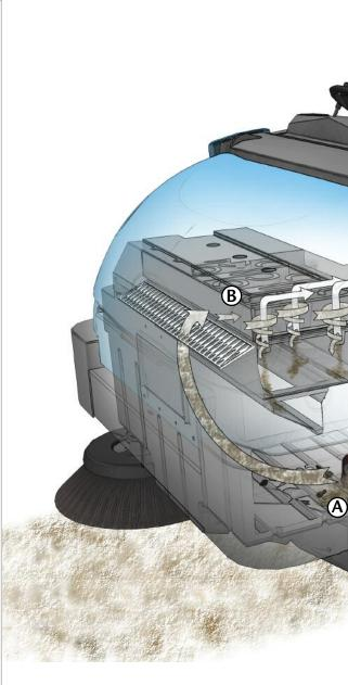
Ensure operator safety, by alerting and shutting down sweeping functions, if increases in hopper temperature are sensed by Thermo-Sentry."
