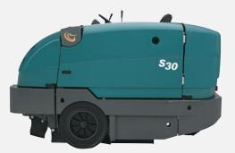
Engineered, fiber-reinforced composite covers are light weight, corrosion resistant, and manufactured with a high-density material. The superior finish makes these covers easy to clean and restorable even if damaged.
